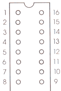
Figure D-8 Internal game connector pin-outs
